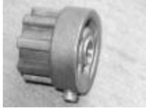
Remove the inching knob from the 1:1 shaft using a small screwdriver. Push the coupler onto the shaft. There is a 5mm brass insert inside the ¼" coupler which will adapt it to the Arri shaft size. Tighten the setscrew on the coupler (1/16" hex wrench). Don't make it too tight or you might raise a burr on the shaft that will make it difficult to remove the coupler.
